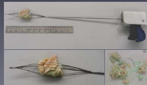
Figure 4: Validation setup (top) with expanded views of basket with simulated gallbladder before (left) and after testing (right).
